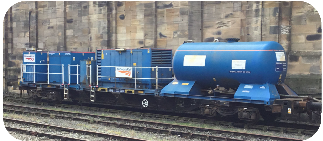
Traction gel application from specialist vehicles
